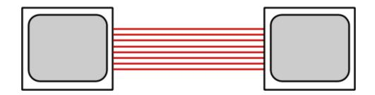
The more lines that a parallel communication medium uses, the more data can be transferred simultaneously.
